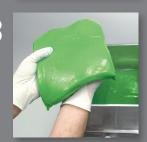
Place up to four gel squares into the Gel Cutting Device hopper.
