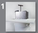
Set up the Gel Cutting Device on the Cutting Board placed over a bucket or storage container.
