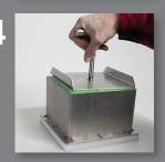
With the Gel Cutting Device plunger, push the gel squares through the blade assembly.
